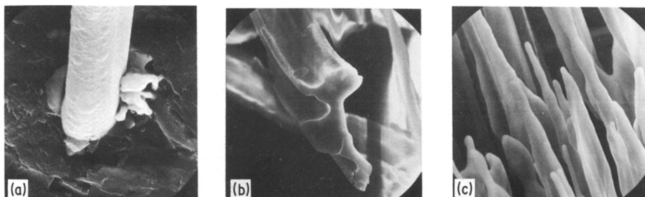
Figure 2 SEM micrographs of (a) root of \text{Pb}(\text{NO}_3)_2 whisker, \times 5400 ; (b) cross-section of \text{KNO}_3 whisker, \times 10000 ; (c) tips of \text{Pb}(\text{NO}_3)_2 whisker, \times 2000 .
